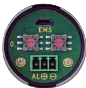
Thermalert 4.0 supports 2-wire loop
