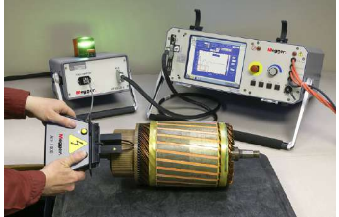
The Baker ZTX in use with the Baker AWA-IV and the ATF5000 commutator test accessory
