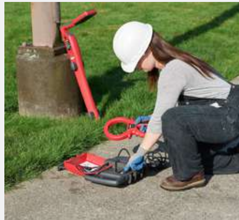
The Transmitter will automatically change modes based on which accessory is plugged in
