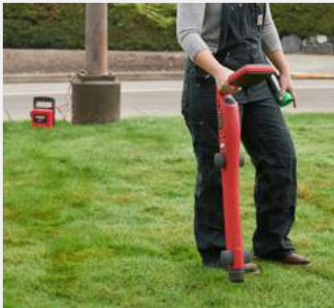
Trace an individual utility by connecting the transmitter directly with the test leads
