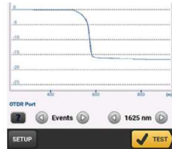
Splitter as seen on an OTDR trace
