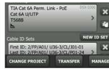
Project specific screen shows up to the minute project details
