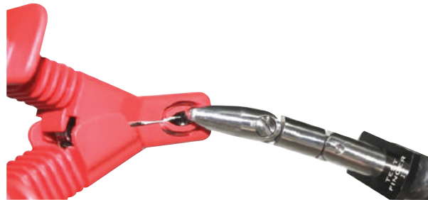
Megger clip being tested with IEC standard test finger for creepage and clearance.
