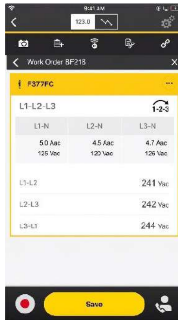
Fluke Connect pulls all data related to three-phase measurements including phase rotation and presents the full set of data for analysis at a glance.
